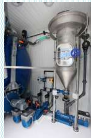
ExSep separator for wastewater pre-treatment before membrane modules
